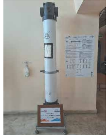
Hollow Fiber Membrane Example used in wastewater treatment brought to the attention of YTU Students and stakeholders.
